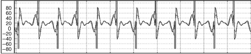
FIGURE 6.12 Voltage of the single-phase series active filter based on the actual method and GSSA method.
